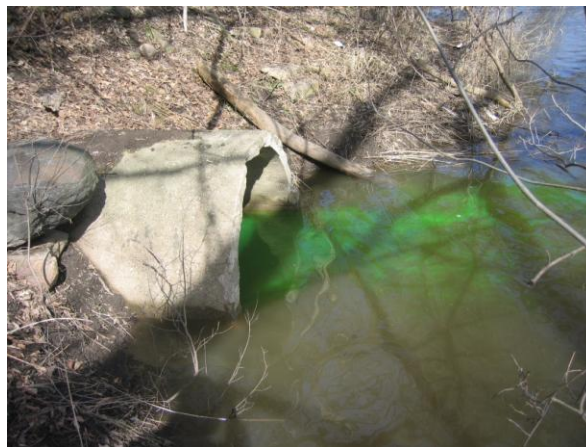
Figure ES-4. Fluorescein dye, which was introduced into sanitary facilities within Miller Park, was released through a stormwater outfall on the Menomonee River.
