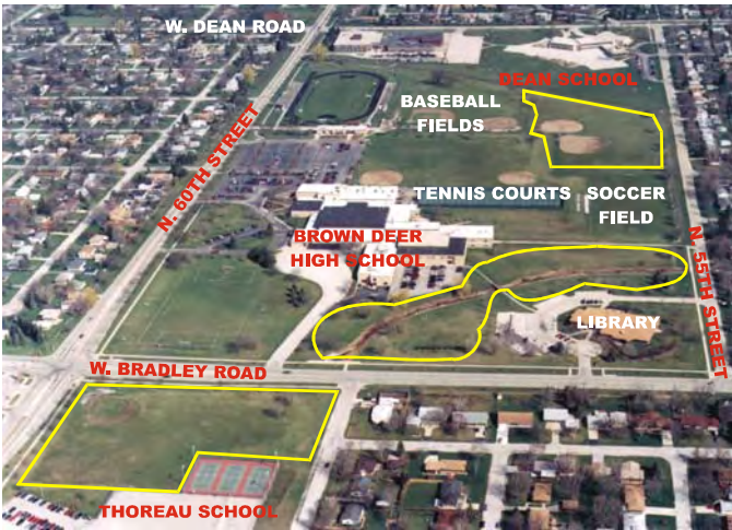
Figure 2 - Planned Detention Basins
